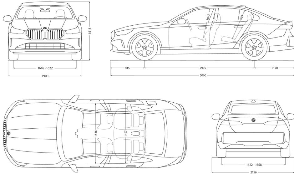
The dimensions in the technical drawing are in millimetres and may vary depending on the model and the optional equipment.
